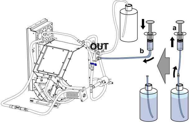
Image 2-8 Filling cooling liquid circuit
